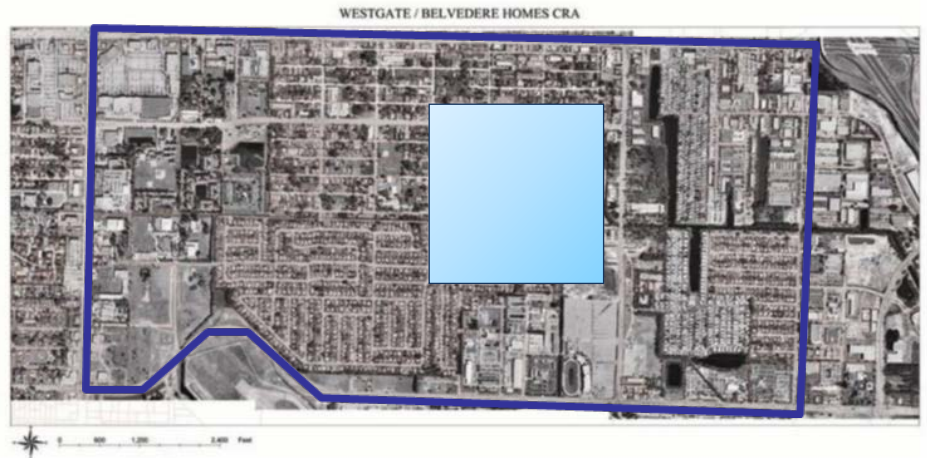
Fig. 2. The blue square superimposed over an aerial photo of the CRA represents an area of about 200 acres, or 15% of the total 1300 acres contained within the CRA. In an ideal situation, this is something close to the area of water retention needed to properly address the current flooding problem.
